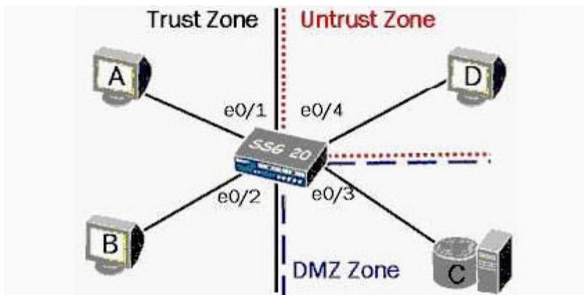
You work as an administrator at Certkiller .com. Study the exhibit carefully. In the exhibit, to enable interface-based NAT between Host A and Host D, which interface(s) must be in NAT mode?
