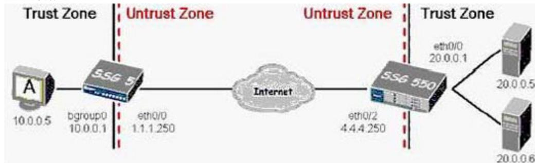
You work as an administrator at Certkiller .com. Study the exhibit carefully. In the exhibit, you need to make a bidirectional gateway between the SSG 5 and the SSG 550. Which gateway address will you configure on the SSG 550 for the VPN?
